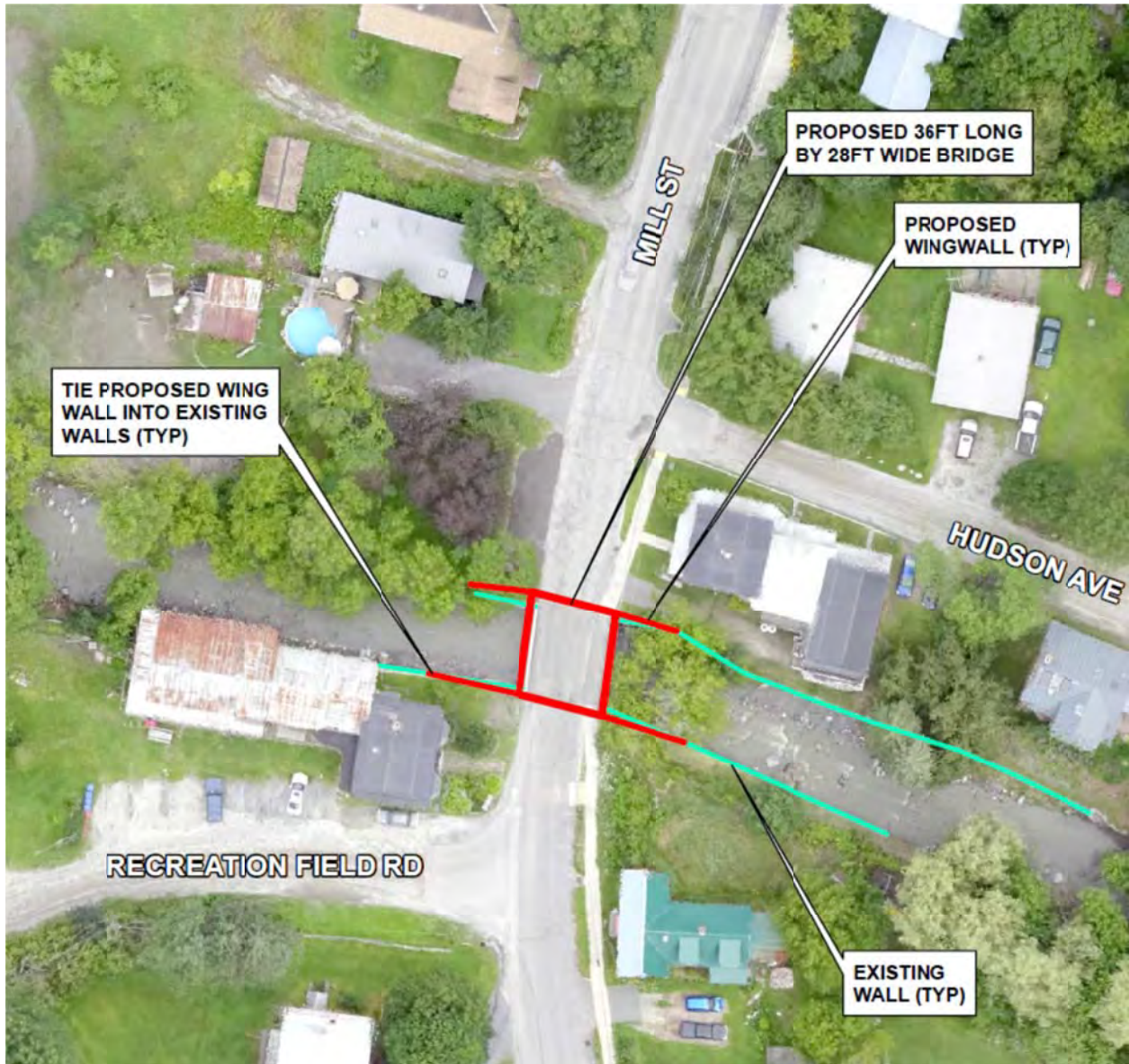
Figure 17: Mill Street Bridge Concept Design
