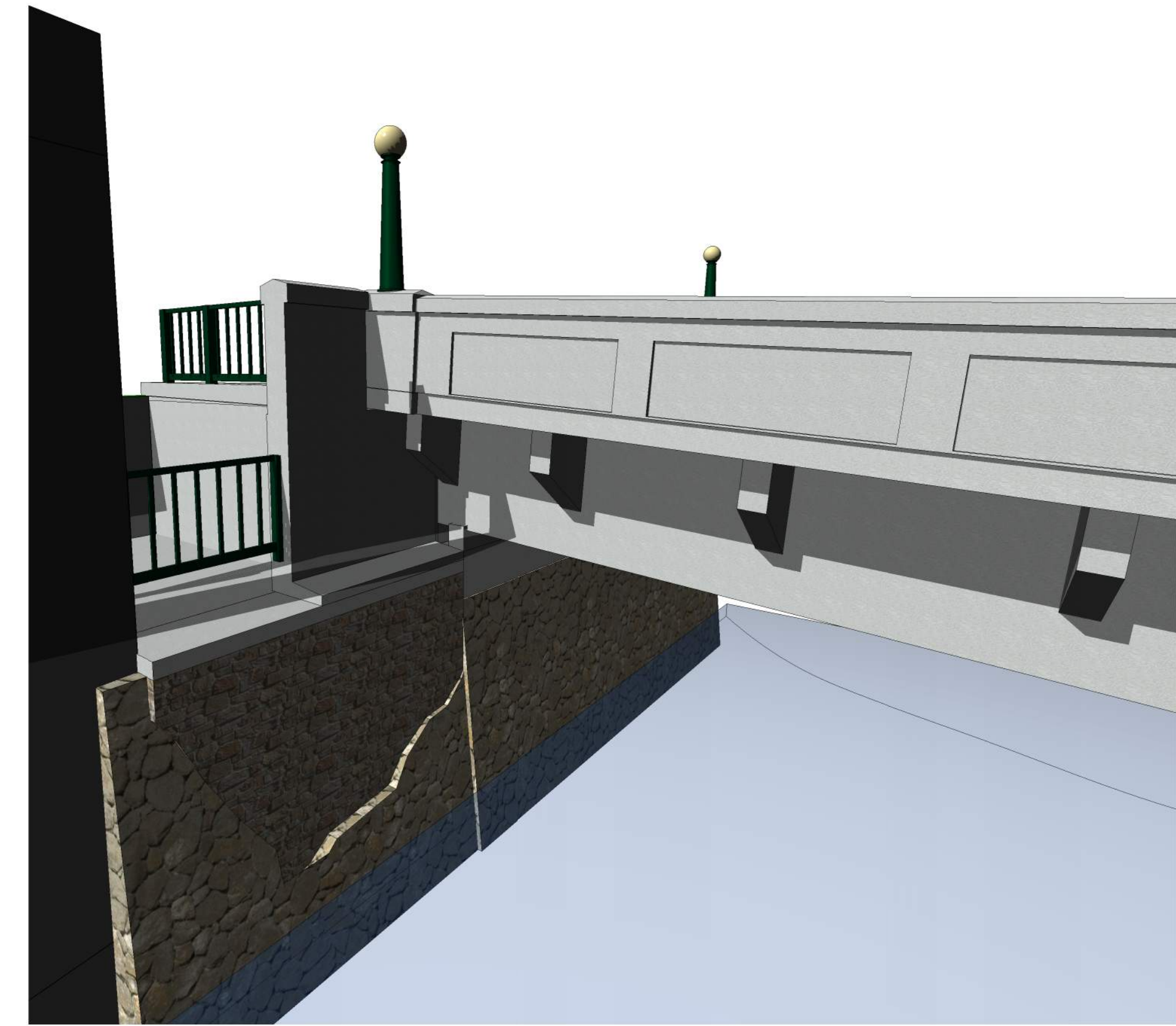
② NEW WEST ABUTMENT
